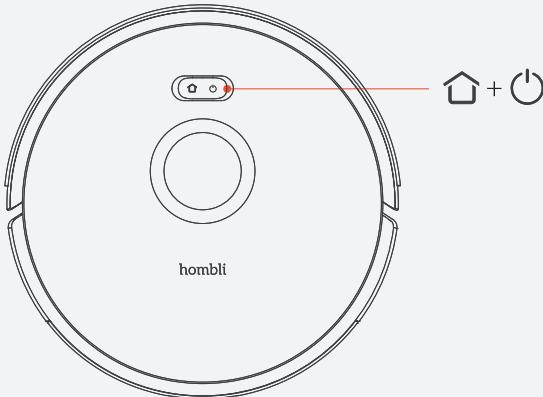
**3.6 Press and hold the home and on/off button for 3 seconds until a white light starts to flash around the buttons**
