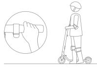
DO NOT press the throttle when walking with the scooter.
